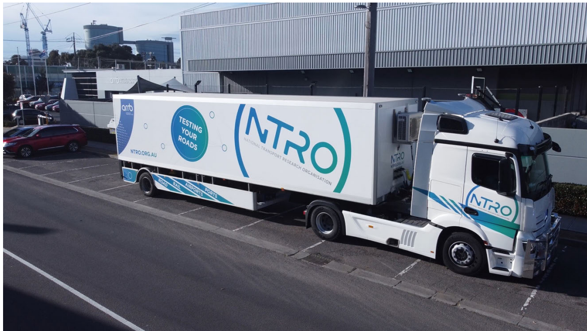
Figure 1 – Intelligent Pavement Assessment Vehicle (iPAVE)
